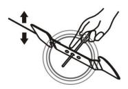
The blade is made of hardened steel. To get a clean job, sharpen the blade frequently, about every 25 hours of use. Make sure the blade is always well balanced.
